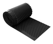
**Foundation foils FK 400** are designed for vertical insulation of foundations, walls and ceilings. The embossing help to keep an air gap which works as insulation, drainage and ventilation.
